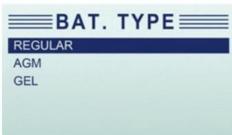
7. Scroll with the UP or DOWN button to select BATTERY STANDARD and press ENTER to confirm. Not all rating systems are available for each application.
