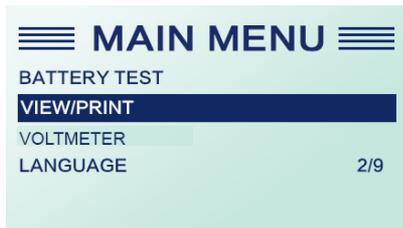
2. Review the test results on the screen. Use the UP or DOWN button to scroll back and forth through Battery Result, Charging Result and Cranking Result to view.
